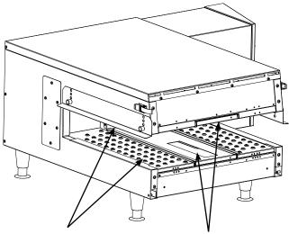
Four impingement jet plates, one in each corner of the cavity, top and bottom
