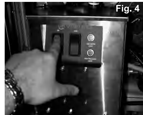
3. AUTOMATIC - After unit is pre-heated, cycle the power switch to the OFF position then immediately back to the ON position.
