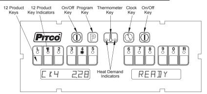
Note 1: Use Left [I/O] key for left side and Right [I/O] key for the right of dual vat control. Use either key on the single vat controller.
