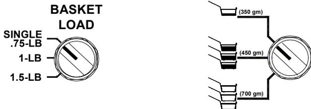
**Position #1:** Single basket loading. Press the Start/Reset Button to dispense a single basket of Fries. Pre-set to .75 lb./350 gm/Single mode.
