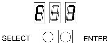
**NOTE:** If you leave the display in this mode, it will return to Normal Operation after a few seconds. This is a safety feature, to prevent functions from being selected by accident.
