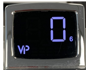
Machines after Serial Number xxxxx3176 display programs as numbers 1-6 instead of as squares.
