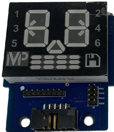
2.3523—Digital Shot Timer Control Board with LED Digits, (Housing and Cover Not Included)
