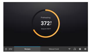
Figure 6: Oven Controls: OneTouch Preheat
