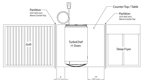
Figure 2: Installation Near Open Heat Source
