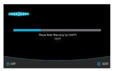
NOTE: When the oven is done warming up, it will "soak" for an additional eight minutes. "Soaking" ensures the cavity surfaces absorb enough heat so that cooking will not be affected.
